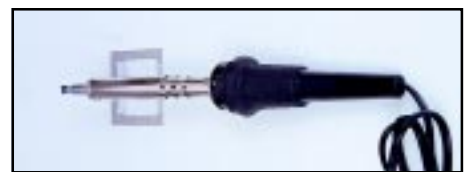
Irons with ceramic heaters.
