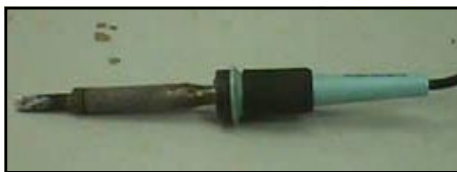
Irons with temperature controlled tips.
